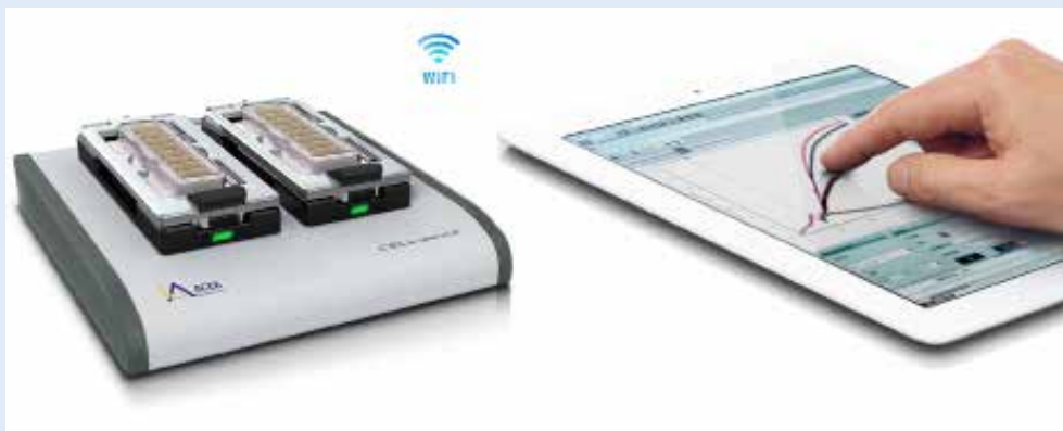
Figure 1. The iCELLigence System. The station houses two E-Plate L8 devices and transfers data via Wi-Fi to the iCELLigence Control Unit for analysis. The E-Plate L8 devices contain 8 wells each with an electrode grid area at the bottom for impedance-based measurements and a view area for microscopic analysis. The Control Unit of the iCELLigence System controls the experimental setup, displays the data in real time, and serves as a platform to perform data analysis.
